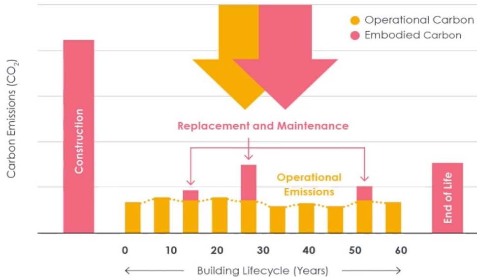
Figure 1 – Building Lifecycle Embodied Carbon. Source: Elementa Consulting .
